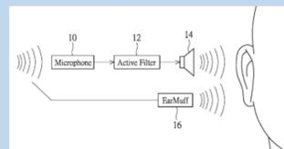
Figure 3: Simplified Headphone Apparatus
