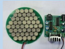
Figure 7: Ultrasonic drivers in parametric series attached to processor
